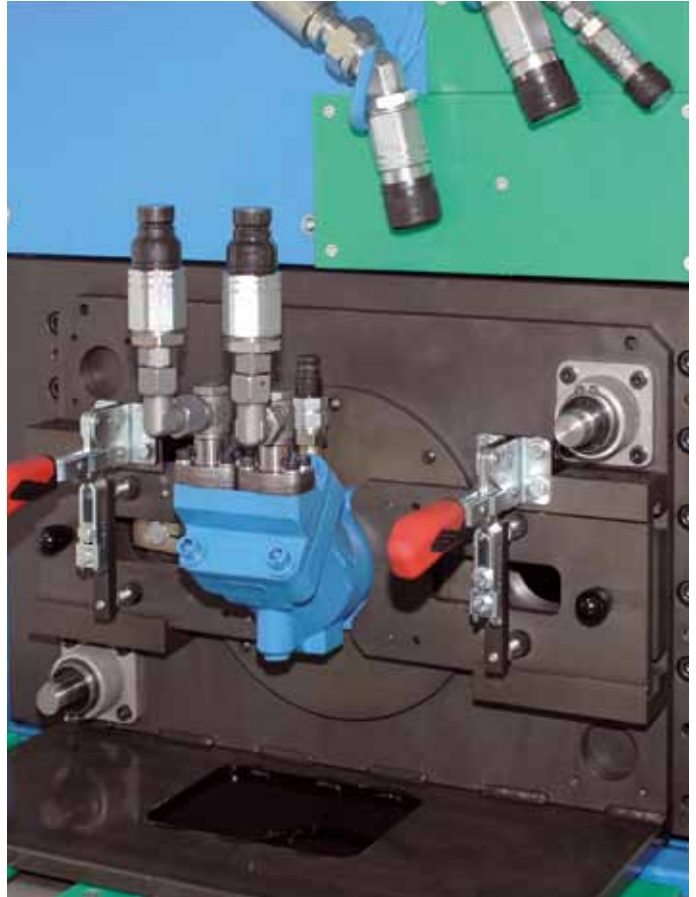
test bench for motors
