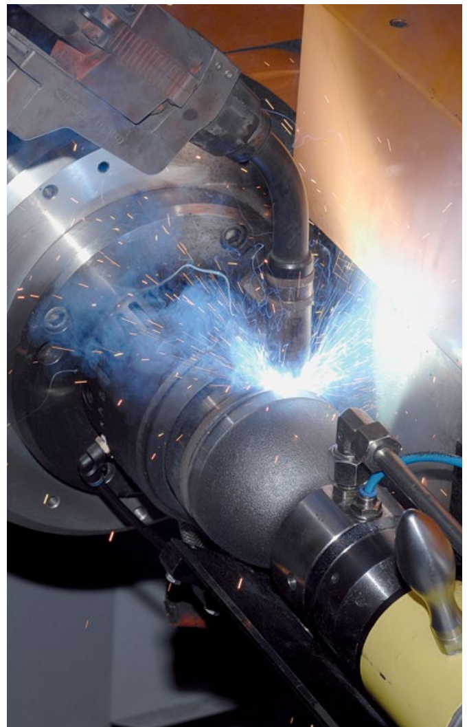
Welding robot for accumulators
